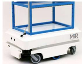
FIGUR 1 - MIR100 FRA MOBILE INDUSTRIAL ROBOTS
